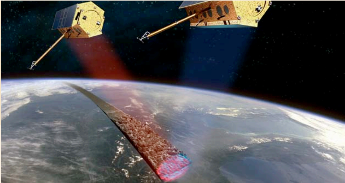
German Earth observation satellites TerraSAR-X and TanDEM-X provide data used to generate a 3-dimensional digital elevation model of unique quality. These data are also used for commercial purposes.
